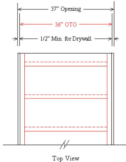
The maximum width of the staircase in this diagram is 36". Due to wall variation, stairs should be ordered 1/4" less than the actual maximum dimension. In this example the out to out dimension would be 35-3/4".
